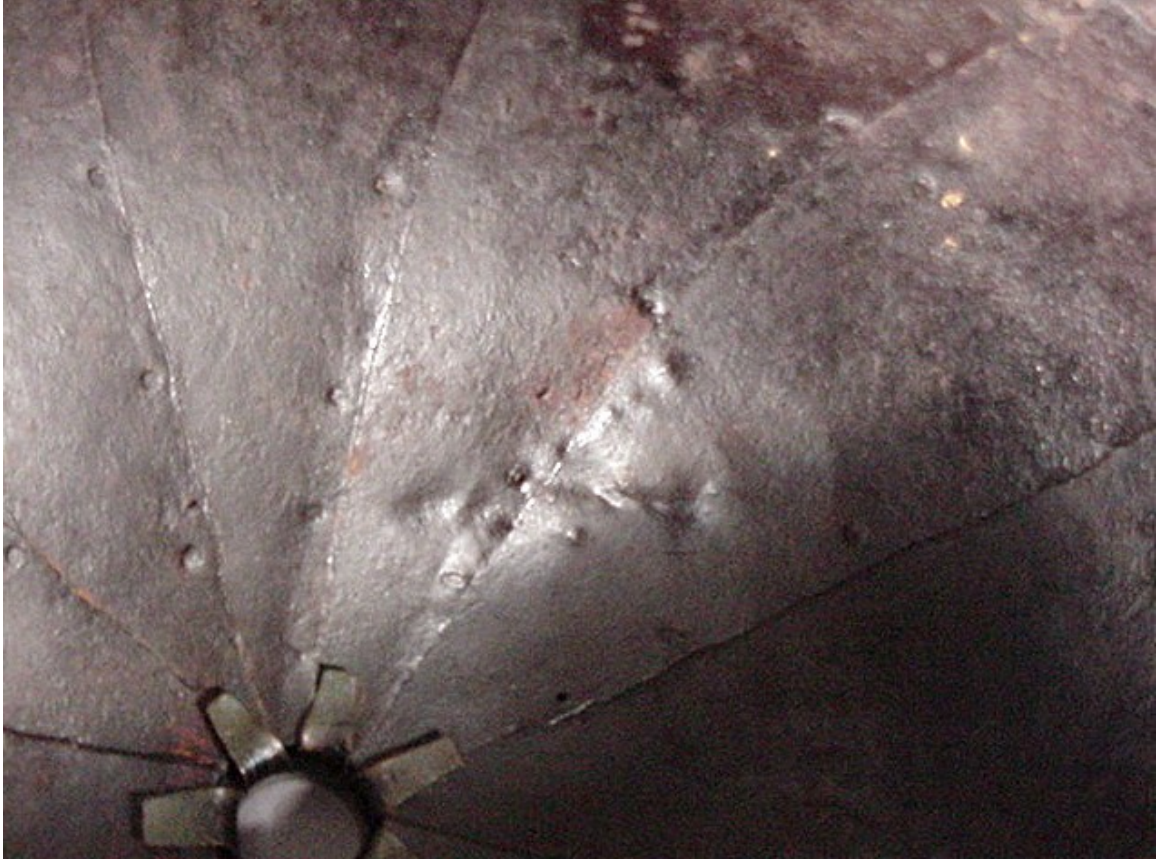
This dent crosses over two plates in this Muromachi era Haruta akoda nari kabuto. The blow was so strong that it knocked out two rivets from the plates. The blow resulted in a significant dent, but the plates were not penetrated. . The metal integrity held, however the shape had to be fixed by building it up with lacquer to make the dent unnoticeable.
